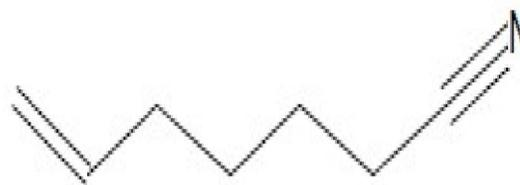
Figure 5.11: Molecular structure of Hept-6-ene nitrile
