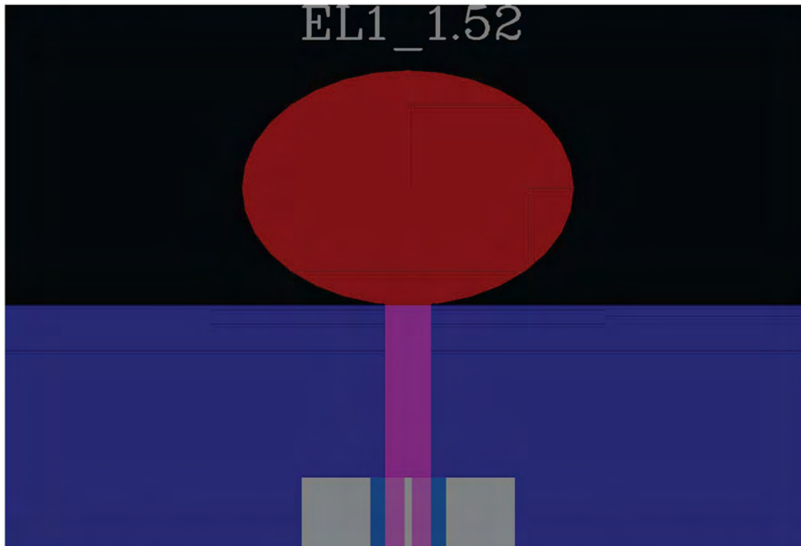
Figure 11. Geometry of the 1.52mm TLY-5 Substrate Elliptic Antenna with solder mask
