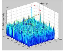
Figure 5. Plot of cross-correlation  $R_l(k)$  of Wibro OFDM signal (FFT size 1024 and CP 128) corrupted through 0dB AWGN.
