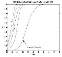
Figure 12. ROC curve for accurately estimated CP length (128) verses channel noise (dB) by varying number of frames.
