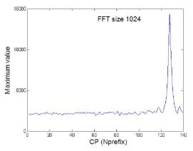
Figure 8. Plot of estimated CP vector for FFT size 1024.
