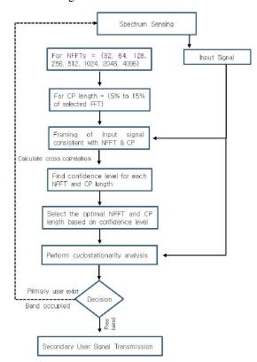
Figure 2. Flowchart of the proposed procedure to estimate.
