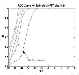
Figure 11. ROC curve for estimated correct FFT size (1024) verses channel noise (dB) by varying number of frames.
