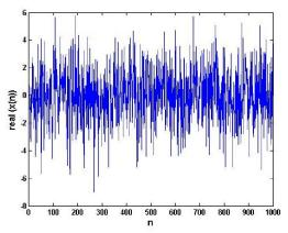
Figure 4. Plot of real coefficients of simulated Wibro OFDM signal corrupted through -5dB AWGN.
