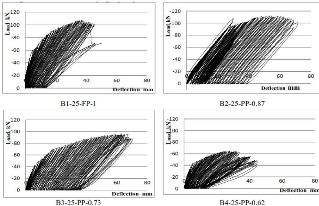
Fig. (8). Hysteresis (P-Δ) curves of beams
