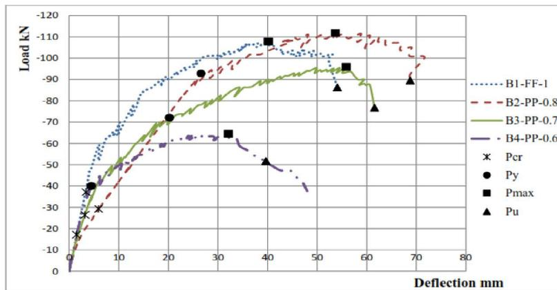
Fig. (7) Total load versus the mid span deflection of all the tested beams.
