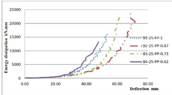
**Fig. (10) Measured energy dissipation capacity of tested beams.**
