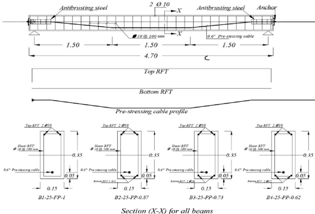
**Fig. (1) Reinforcement details of specimen's**
