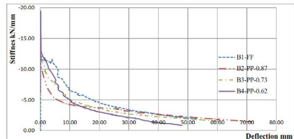
**Fig. (9) Stiffness degradation of all tested beams**
