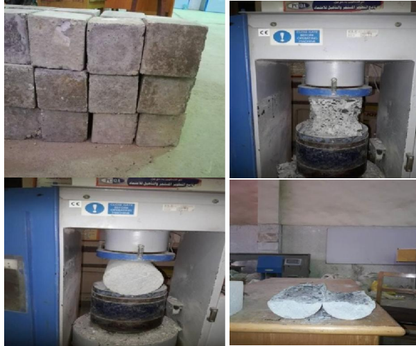
Figure. 4: Compressive and Splitting tensile tests
