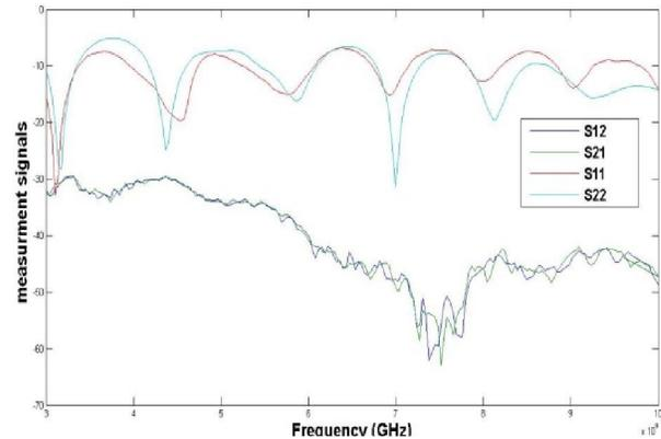
Fig 4: - The measurement signals  $S_{11}$ ,  $S_{22}$ ,  $S_{21}$ ,  $S_{12}$  with a vector network analyzer.
