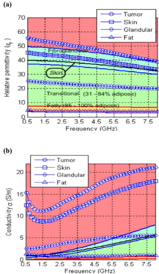
Fig 7:- ( a ) Relative permittivity of phantom materials ( b ) Conductivity.
