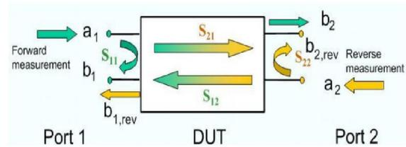
Fig 3: - Signals path  $S_{11}$ ,  $S_{22}$ ,  $S_{21}$ ,  $S_{12}$
