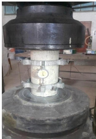
Figure 3. Experimental Set-Up for Modulus of Elasticity Test
