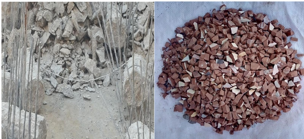
a- Waste Concrete b- Waste ceramic Figure 2. Recycled Concrete Aggregate
