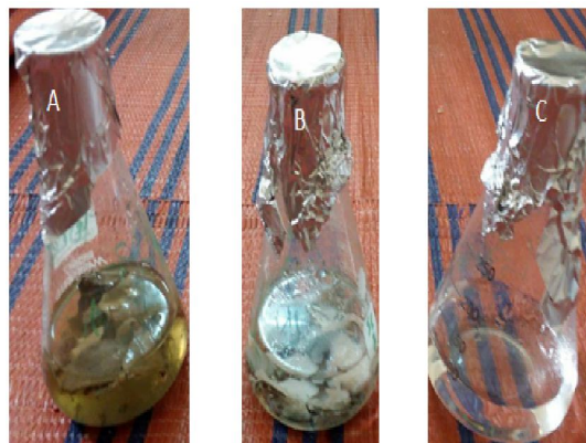
Figure 1. Conversion of silver nitrate to nano silver by A. alternata (A, silver nitrate solution inoculated with fungus biomass; B, distilled water inoculated with biomass of fungus; C, silver nitrate solution without fungus biomass).
