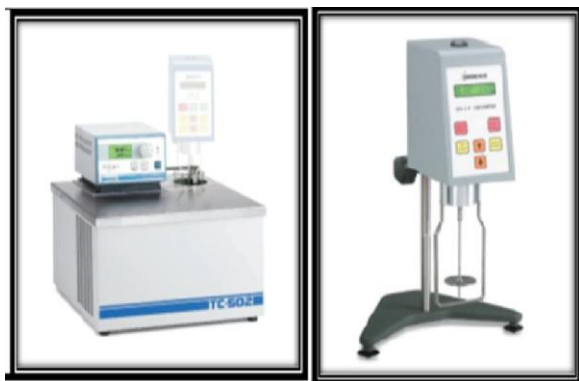
Fig.2: Brookfield viscometer and temperature control to control sample temperature during viscosity measurements.
