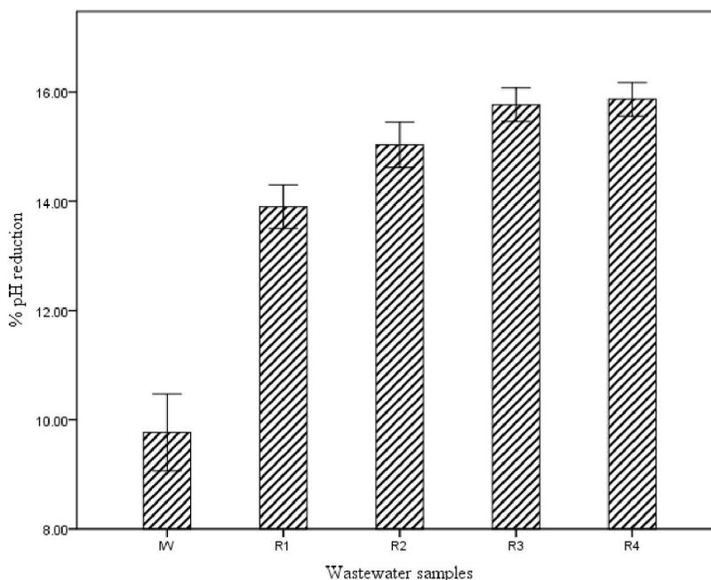
Figure 1. Reduction of pH of textile wastewater after gamma irradiation in presence of H<sub>2</sub>O<sub>2</sub>
