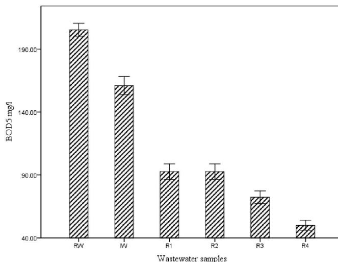
Figure 5. Reduction of  $\text{BOD}_5$  of irradiated wastewater in presence of  $\text{H}_2\text{O}_2$
