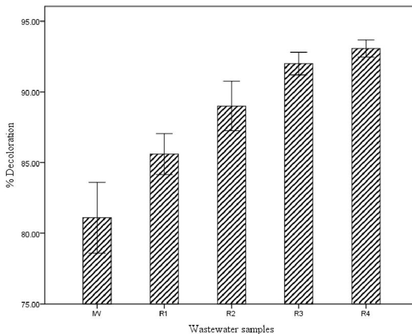
Figure 2. Color reduction (%) of wastewater in presence of  $H_2O_2$  after gamma irradiation
