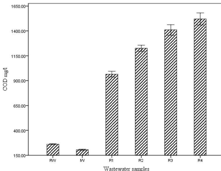
Figure 4. Variation of COD values of gamma irradiated textile wastewater in presence of  $\text{H}_2\text{O}_2$
