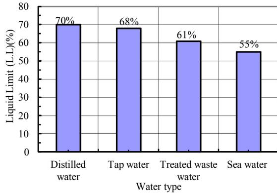
**Fig.7:** Effect of water types on liquid limit
