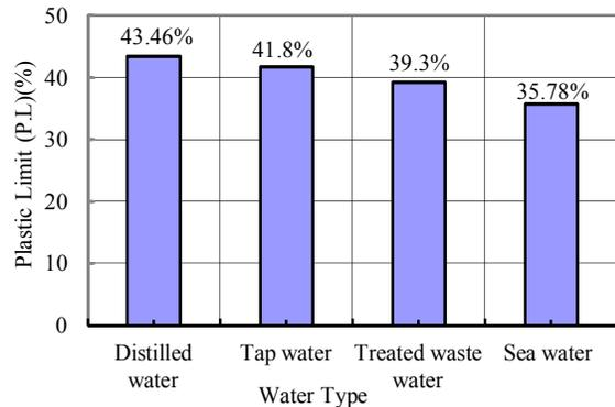
**Fig.8:** Effect of water types on plastic limit
