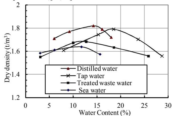
**Fig.10:** Compaction curves for expansive clayey soil using different water types
