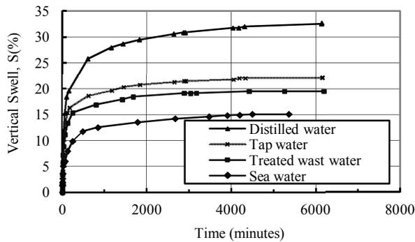
**Fig.2:** Vertical swell percent versus time for different water types(Using Proctor cylinder)
