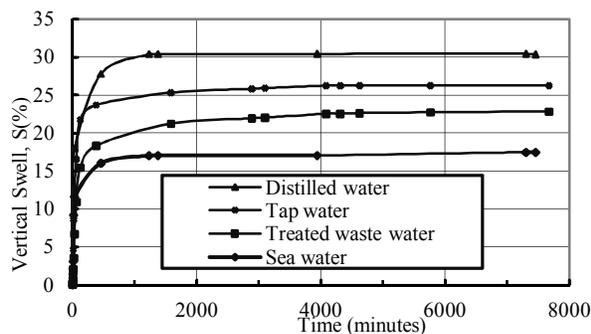
**Fig.3:** Vertical swell percent versus time for different water types(Using Oedometer ring)
