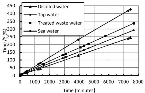
**Fig.5:** Time/S ratio versus time for different water types (Using Oedometer ring)
