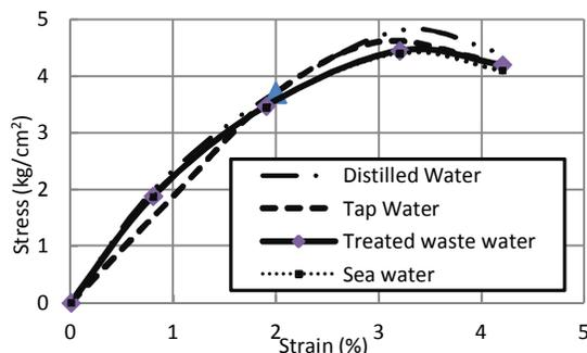
Fig. 11: Results of unconfined compressive strength for expansive clay sample mixed with different water types.
