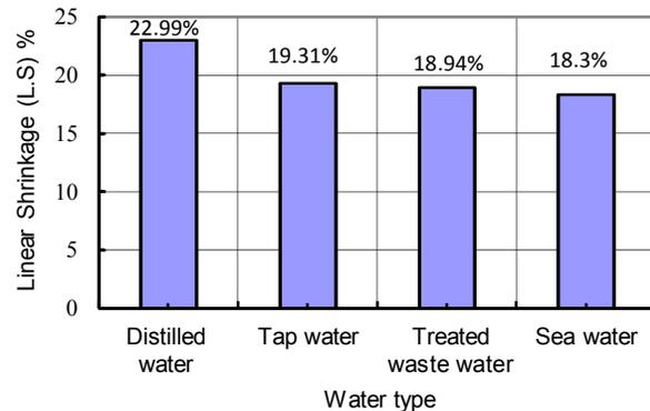
**Fig.9:** Effect of water types on linear shrinkage
