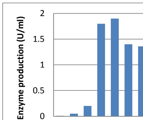
Fig. 4. Effect of different incubation period on PHB degradation (enzyme production, U/ml) by the selected fungal isolate.
