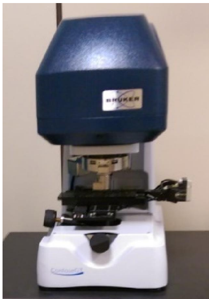
Fig 2: 3D optical noncontact surface profiler
