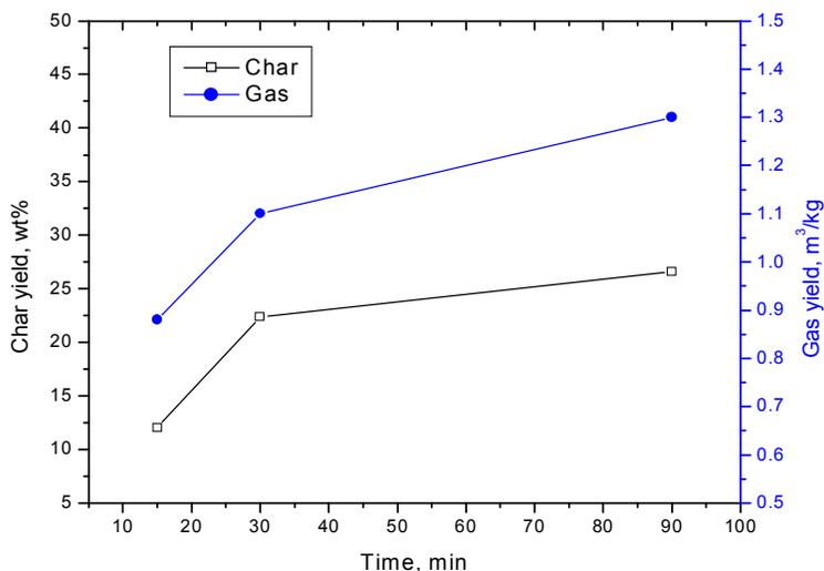
Figure 6. Effect of time of reaction on gasification processes
