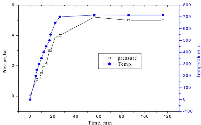
Figure 3. Profile of temperature, pressure against time of reaction during gasification
