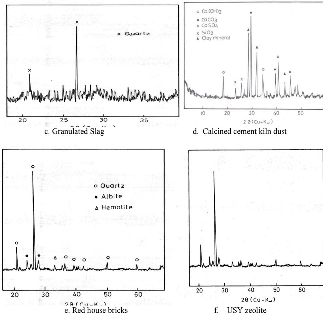
Figure 1. XRD of different catalysts used in gasification of saw dust
