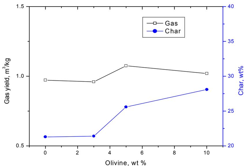
Figure 9. Effect of olivine catalyst on the gasification processes
