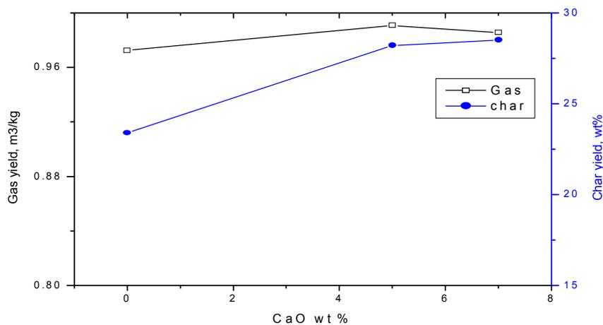
Figure 16. Effect of CaO on gasification of saw dust
