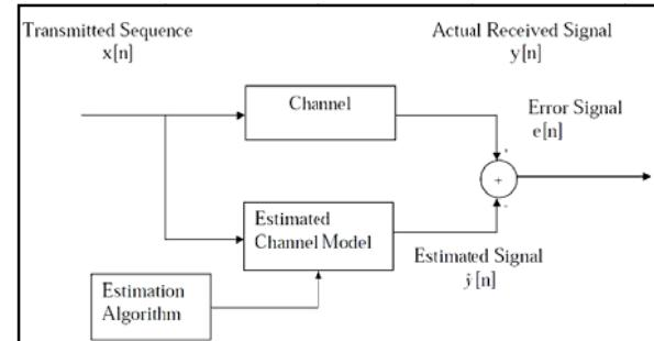
Figure [2]: block diagram for channel estimation [2]
