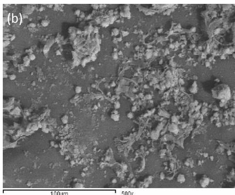
**Figure 5:** SEM of (a) tosyl methyl cellulose loaded with the anti-acid and (b) trimethylsilyl methyl cellulose loaded with the anti-acid
