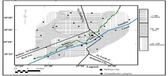
Fig. (9): Total Hardness (TH) zonation map of the Quaternary aquifer samples, Belbies district, categories classified for laundry uses according to Durfer and Becker (1964).
