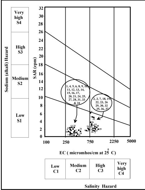
Fig. (10): Classification of the studied groundwater samples for irrigation, Belbies district (based on U.S. Salinity Laboratory Staff, 1954).
