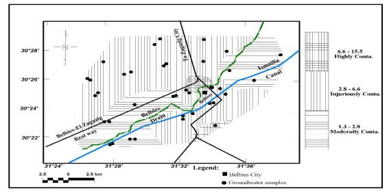
Fig. (3): Zonation map of the (Cl/(HCO<sub>3</sub>+CO<sub>3</sub>) ratio of the Quaternary groundwater in Belbies district.
