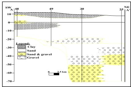
Fig. (2): Geological cross section along the direction A-A' (wells data after Research Institute for Groundwater "RIGW", 1980).
