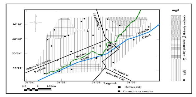
Fig. (7): Nitrate (NO<sub>3</sub>) zonation map of the Quaternary aquifer samples at Belbies district, categories classified for drinking uses according to Kumar *et al.* (2002) and Thorburn *et al.* (2003).
