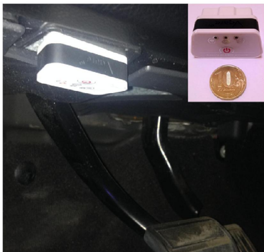
Fig. 2. Example of connecting the device with chip ELM327 to the vehicle
