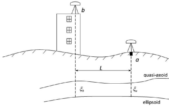
In this case, geodetic heights  $h_{g_a}$  and  $h_{g_b}$  of points  $a$  and  $b$  are defined as the sum of normal heights  $h_{h_a}$  and  $h_{h_b}$ , and heights of the quasi-geoid above the reference ellipsoid
