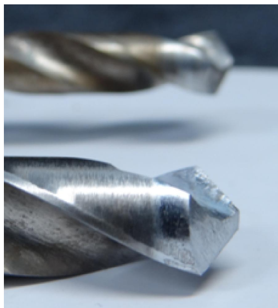
Fig.4. Overview of drills with locally strengthened cutting zone
