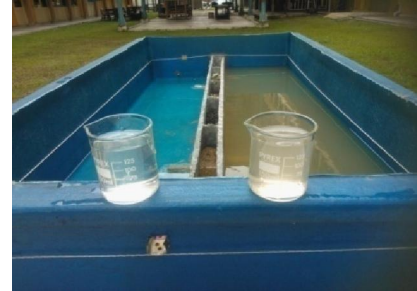
Fig.9- The effect of channel partition in TSS removal efficiency before and after the channel
