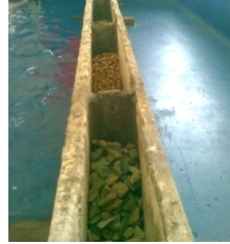
Fig 6- Stratified sand filter in channel partition
