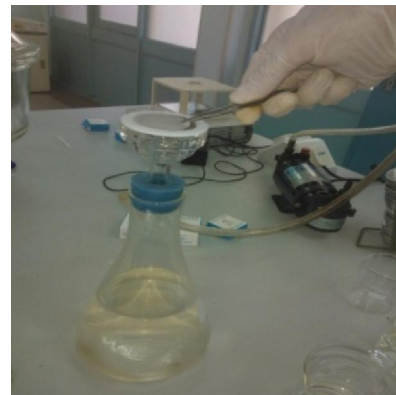
Fig-7- TSS measurement in UTM laboratory
