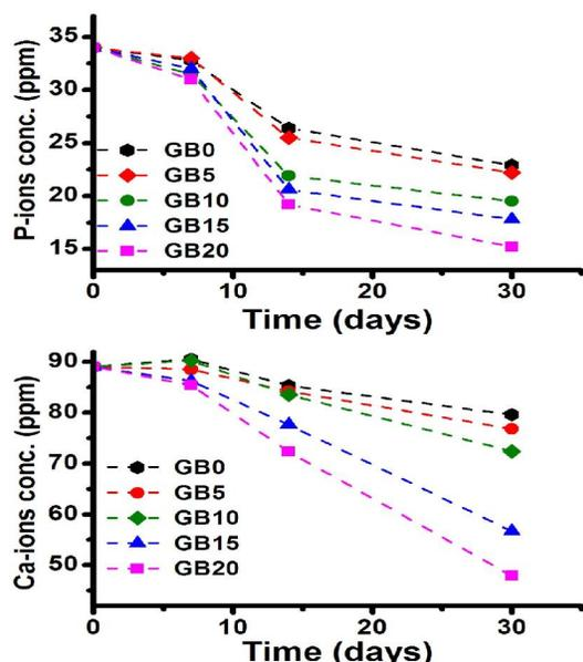
Fig (11). Variation of P- and Ca-ions concentrations in the SBF solution after soaking of the studied glasses for 7, 14 and 30 days.
