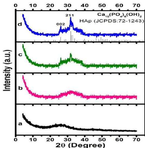
Fig. (1) XRD patterns of glass GB20: a) as-prepared sample; b-d) after soaking the glass in SBF for 7, 14 and 30 days, respectively
