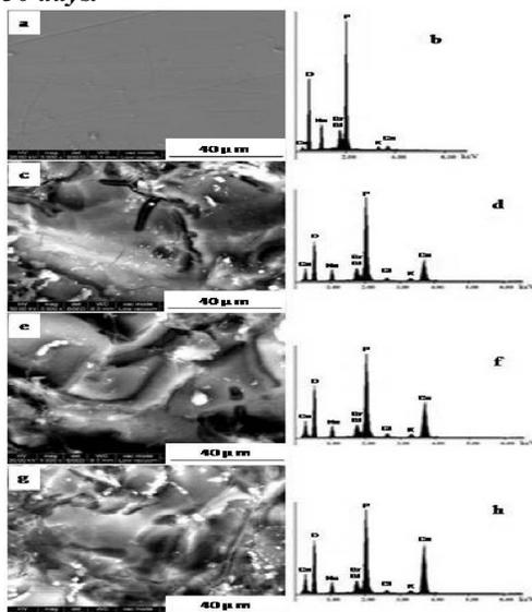
Fig (8): SEM micrographs and the corresponding EDAX spectra of glass GB10: a, b) as-prepared glass, i. e. before immersion in the SBF; c, d) after immersion in the SBF for 7 days; e, f) after immersion in the SBF for 14 days; g, h) after immersion in the SBF for 30 days.
