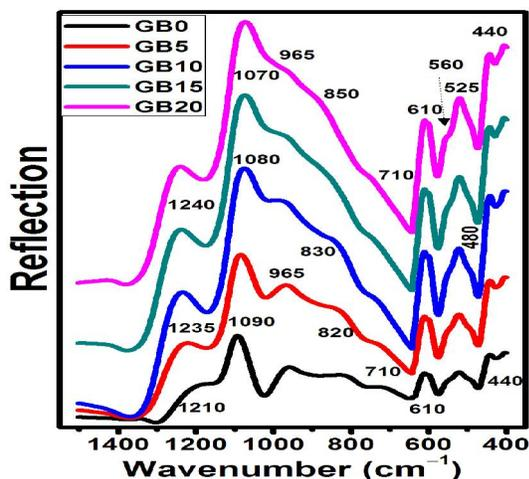
Fig(3): FTIR spectra of the investigated glasses after soaking in the SBF for 7 days.
