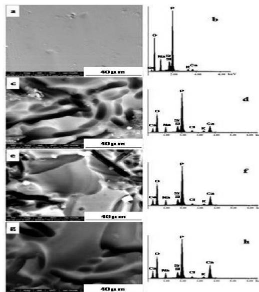
Fig(6): SEM micrographs and the corresponding EDX spectra of glass GB0: a, b) as-prepared glass, i. e. before immersion in the SBF; c, d) after immersion in the SBF for 7 days; e, f) after immersion in the SBF for 14 days; g, h) after immersion in the SBF for 30 days.
