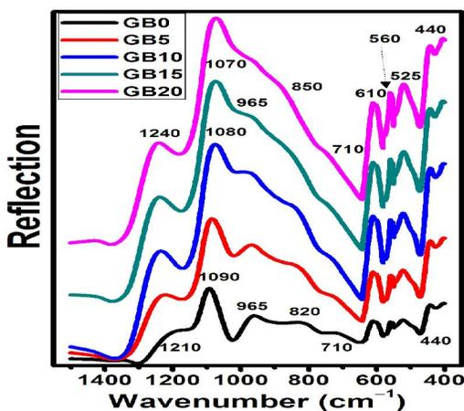
Fig(4): FTIR spectra of the studied glasses after soaking in the SBF for 14 days.
