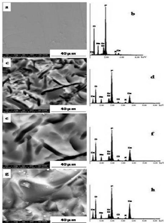
Fig (7): SEM images and the corresponding EDAX spectra of glass GB5: a, b) as-prepared glass, i. e. before immersion in the SBF; c, d) after immersion in the SBF for 7 days; e, f) after immersion in the SBF for 14 days; g, h) after immersion in the SBF for 30 days.
