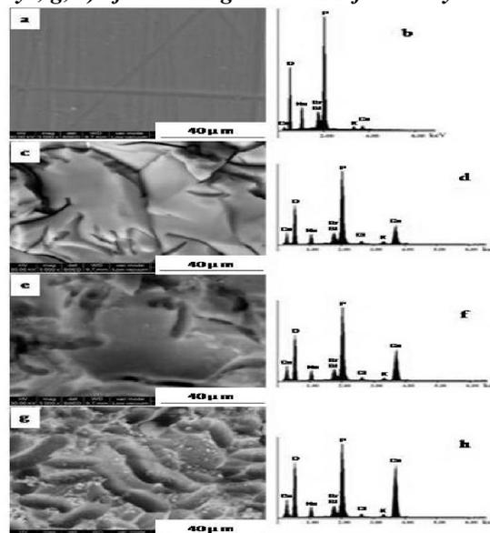
Fig (10): SEM micrographs and the corresponding EDAX spectra of glass GB20: a, b) as-prepared glass, i. e. before soaking in the SBF; c, d) after soaking in the SBF for 7 days; e, f) after soaking in the SBF for 14 days; g, h) after soaking in the SBF for 30 days
