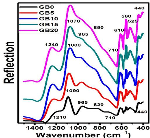
Fig(5): FTIR spectra of the investigated glasses after soaking in the SBF for 30 days.
