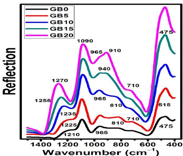
Fig(2): FTIR spectra of the as-prepared glasses, i. e. before soaking in the SBF.
