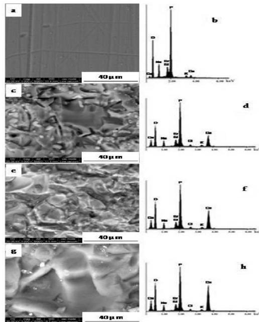
Fig (9): SEM images and the corresponding EDAX spectra of glass GB15: a, b) as-prepared glass, i. e. before soaking in the SBF; c, d) after soaking in the SBF for 7 days; e, f) after soaking in the SBF for 14 days; g, h) after soaking in the SBF for 30 days.
