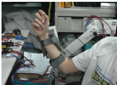
Figure 13. Actual installation diagram of the arm exoskeleton
