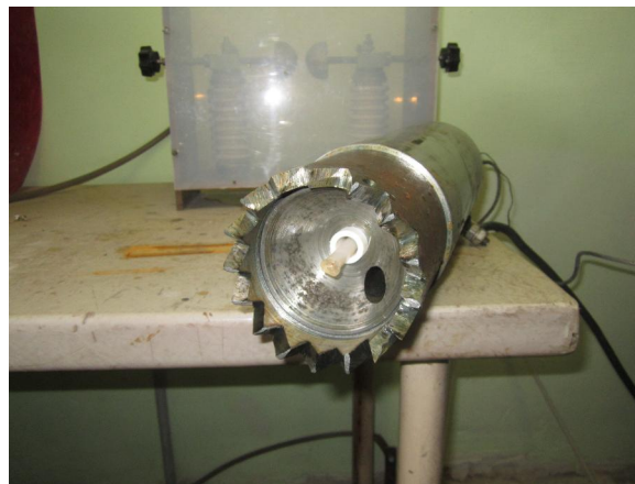
Fig. 2. The appearance of the electro-hydraulic drill
