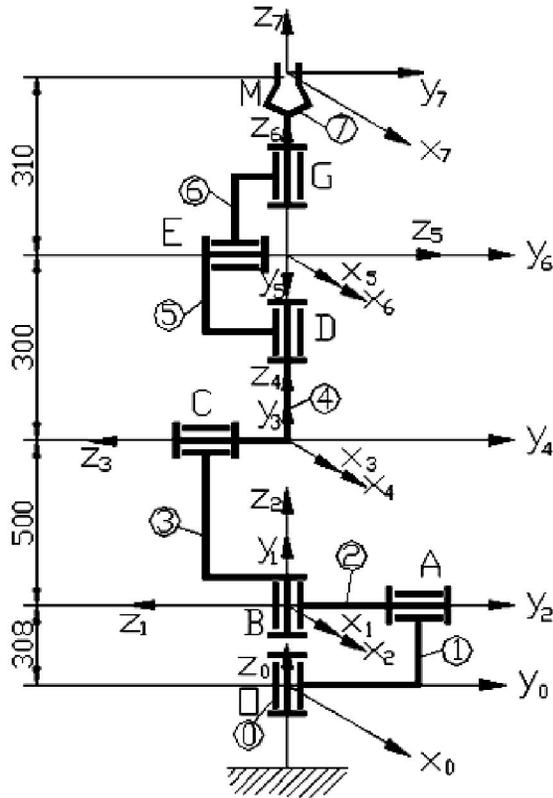
Fig. 1. KS of a medical robot with designated Denavit-Hartenberg coordinate systems
