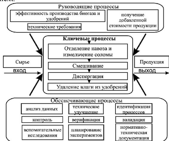
Figure 1 – Flow-process diagram of biogas unit
