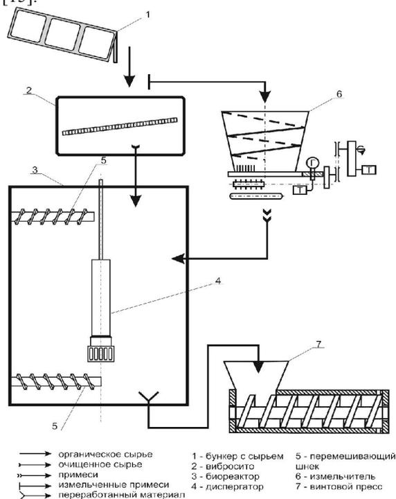
Figure 2 – General process flow diagram of biogas unit functioning
