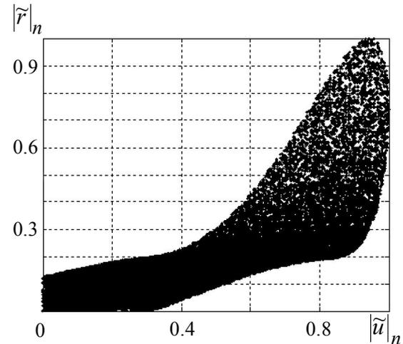
**Fig. 2 Normalized non-linear amplitude characteristic of the PA**
