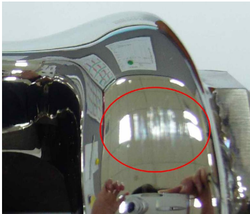
Figure 5(b) Femoral component: after test of 5,000,000 cycles.
