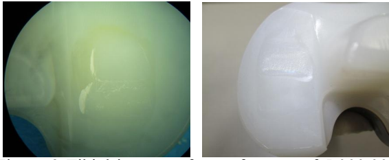
Figure 9 Tibial insert surfaces after test of 5,000,000 cycles (left: not cryo-treated, right: cryo-treated).
