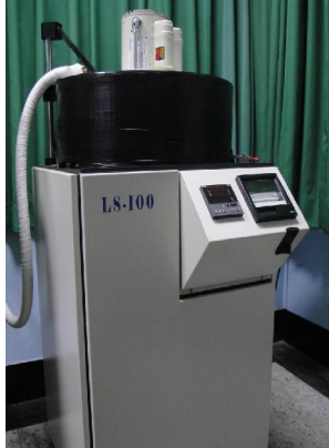
Figure 2 LS-100 Cryogenic Processor.
