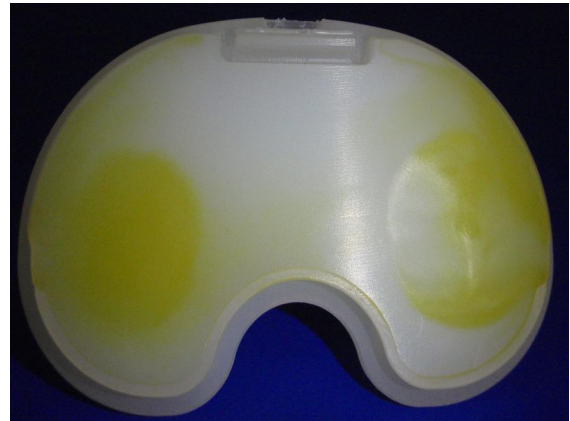
Figure 7 Insert backside surface after test of 5,000,000 cycles.
