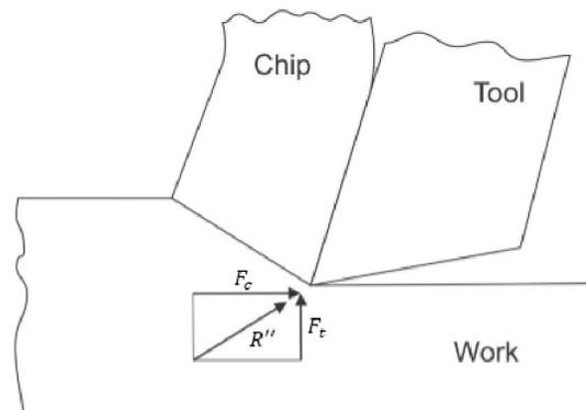
Figure 2: Forces acting on the tool that can be measured (after (Groover 2010))
