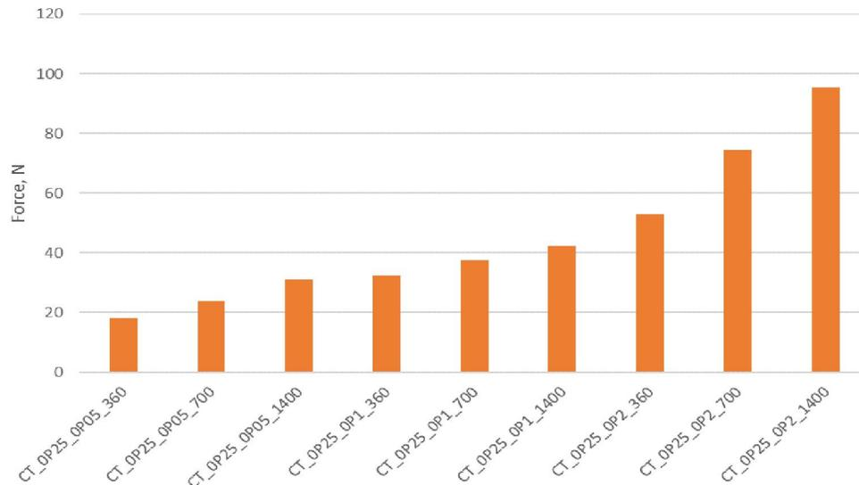
Figure 5: Machining forces as recorded by the force dynamometer for  $d = 0.25$  mm
