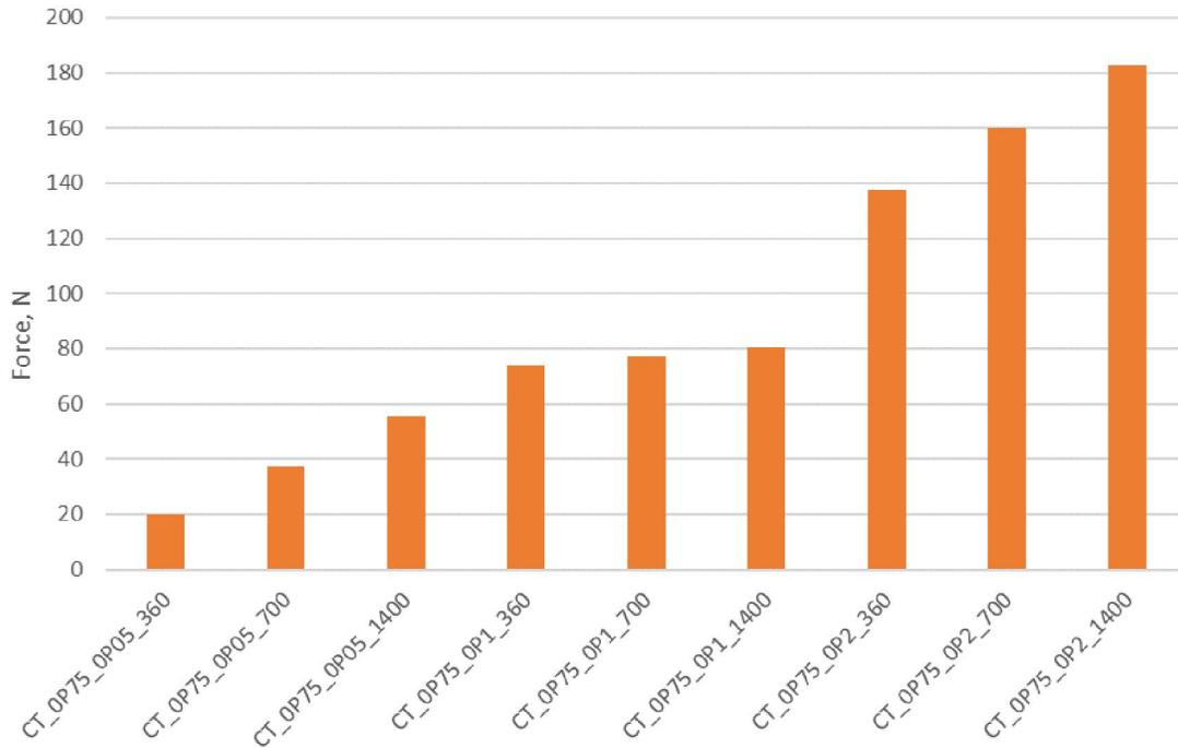
Figure 7: Machining forces as recorded by the force dynamometer for  $d = 0.75 \text{ mm}$
