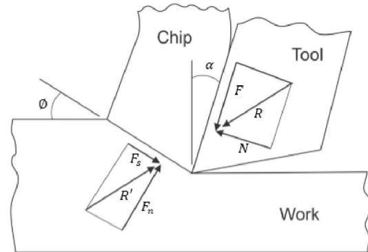
Figure 1: Forces acting on the chip in orthogonal cutting (after (Groover 2010))
