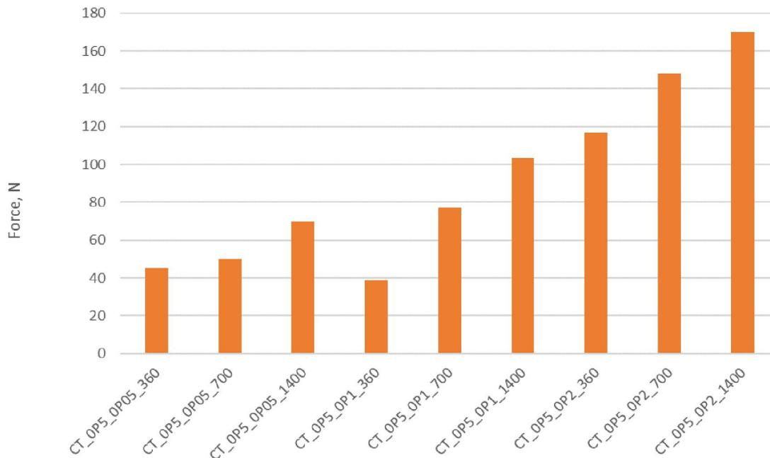
Figure 6: Machining forces as recorded by the force dynamometer for  $d = 0.5$  mm
