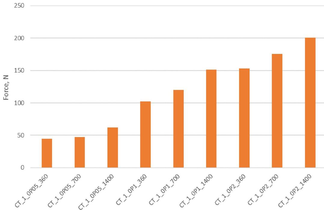
Figure 8: Machining forces as recorded by the force dynamometer for  $d = 1 \text{ mm}$
