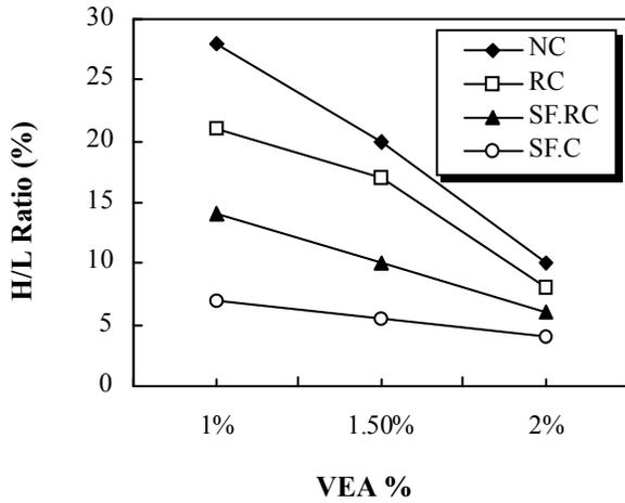
Fig. 9. H/L Ratio of Different Mixes Containing Dolomite Aggregate.
