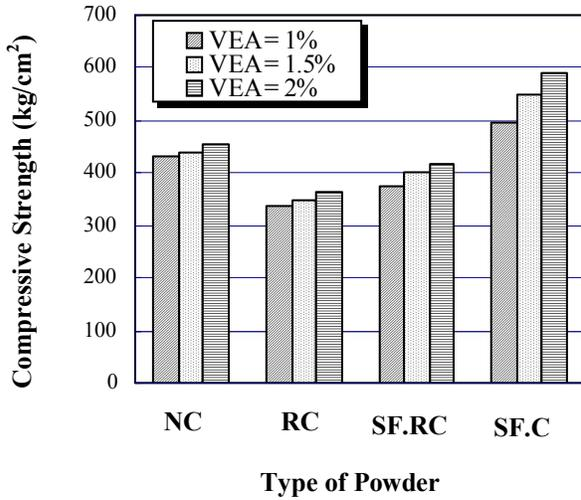
Fig. 11. Compressive Strength of Different Mixes Containing Dolomite Aggregate.
