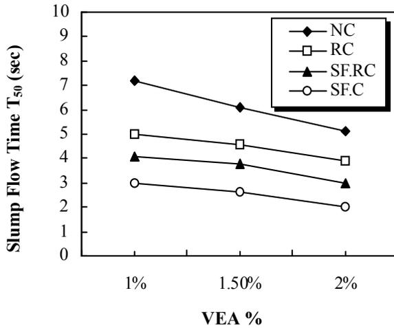
Fig. 5. Slump Flow Time ( $T_{50}$ ) of Different Mixes Containing Dolomite Aggregate.
