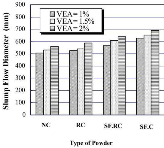
Fig. 3. Slump Flow Diameter of Different Mixes Containing Dolomite Aggregate.
