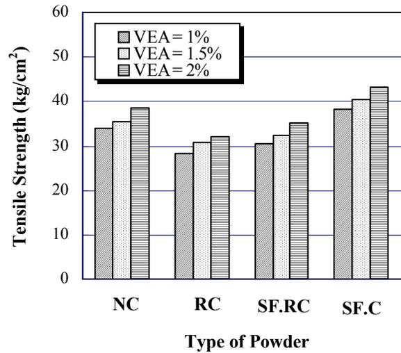
Fig. 14. Tensile Strength of Different Mixes Containing Gravel Aggregate.
