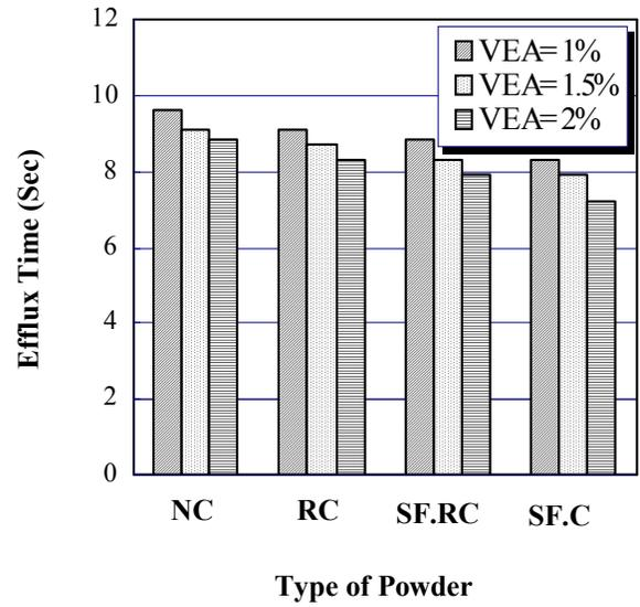
Fig. 8. V-Funnel Flow Time of Different Mixes Containing Gravel Aggregate.
