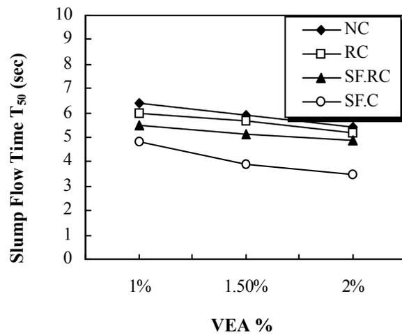
Fig. 6. Slump Flow Time ( $T_{50}$ ) of Different Mixes Containing Gravel Aggregate.
