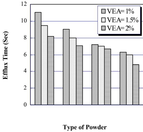
Fig. 7. V-Funnel Flow Time of Different Mixes Containing Dolomite Aggregate.
