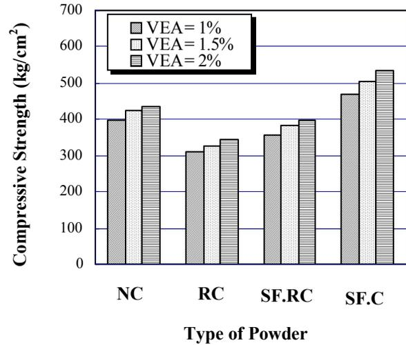
Fig. 12. Compressive Strength of Different Mixes Containing Gravel Aggregate.
