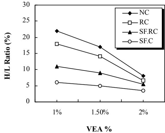
Fig. 10. H/L Ratio of Different Mixes Containing Gravel Aggregate.
