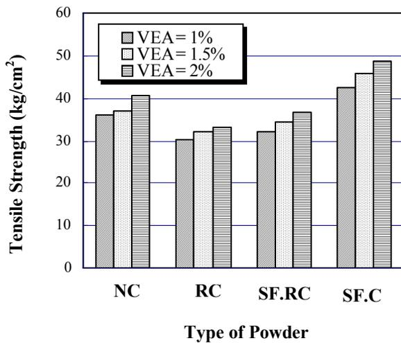
Fig. 13. Tensile Strength of Different Mixes Containing Dolomite Aggregate.
