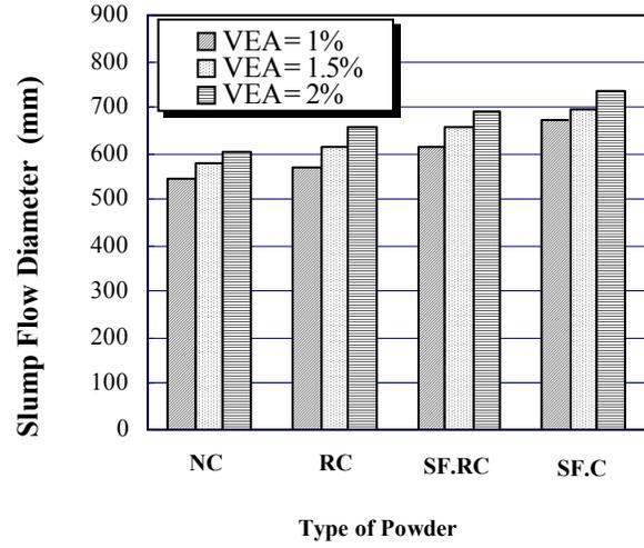
Fig. 4. Slump Flow Diameter of Different Mixes Containing Gravel Aggregate.
