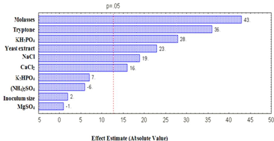
Figure 7. Pareto chart of standardized effects for emulsification index for the Plackett-Burman design. The point at which the effect estimates were statistically significant (at  $p \leq 0.05$ ) is indicated by the broken vertical line.
