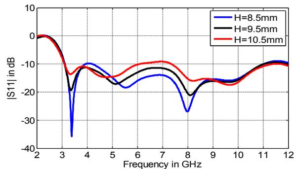
Figure 3. The return loss of the proposed UWB slot antenna at  $B=12 \text{ mm}$ ,  $W_s=18 \text{ mm}$ , and different values of the triangular stub height ( $H$ ).
