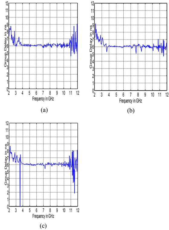
Figure 9. The measured group delay of two of the proposed antenna aligned (a) Face-to-Face, (b) Face-to-Side, and (c) Side-to-Side.
