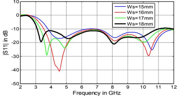
Figure 4. The return loss of the proposed UWB slot antenna at B=12mm, H=9.5mm and different values of slot width (Ws).
