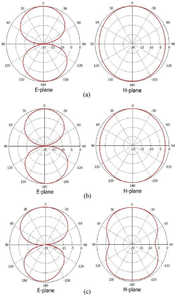
Figure 5. The power pattern of the proposed antenna at (a) 3.36GHz, (b) 5.15GHz, and (c) 8.1GHz.
