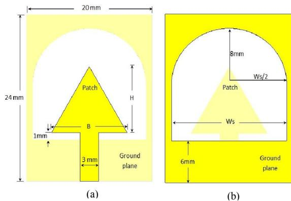
Figure 1. The geometry of the proposed UWB slot antenna (a) front view and (b) back view.
