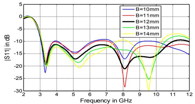
Figure 2. The return loss of the proposed UWB slot antenna at  $H=9.5 \text{ mm}$ ,  $W_s=18 \text{ mm}$ , and different values of the triangular stub base ( $B$ ).
