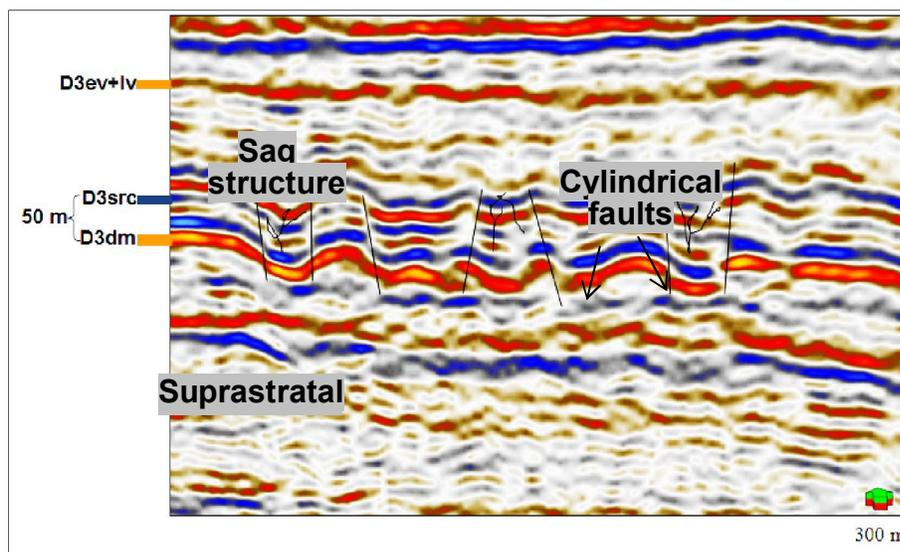
**Figure 6.** Seismic line showing missing sections (collapse in Domanik-Sirachoy section), cylindrical faults, and sag structures.
