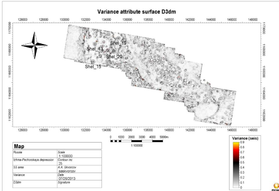
**Figure 5.** Variance attribute time slice showing ring-shaped structures in Domanik formation
