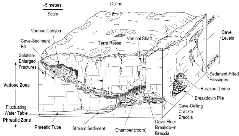
**Figure 1.** The block diagram shows near surface karst terrain with phreatic (below the water table) and vadose (above the water table) cave features. The figure is from Loucks and Handford (1992).
