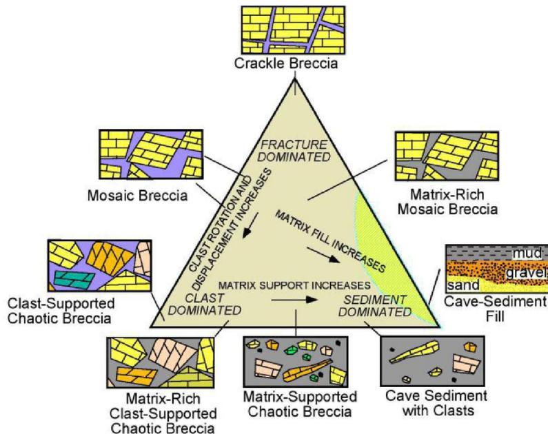
**Figure 2.** Triangle classification showing the breccia and clast deposits within a cave system. Originally from Loucks (1999), modified in Loucks et al. (2007)
