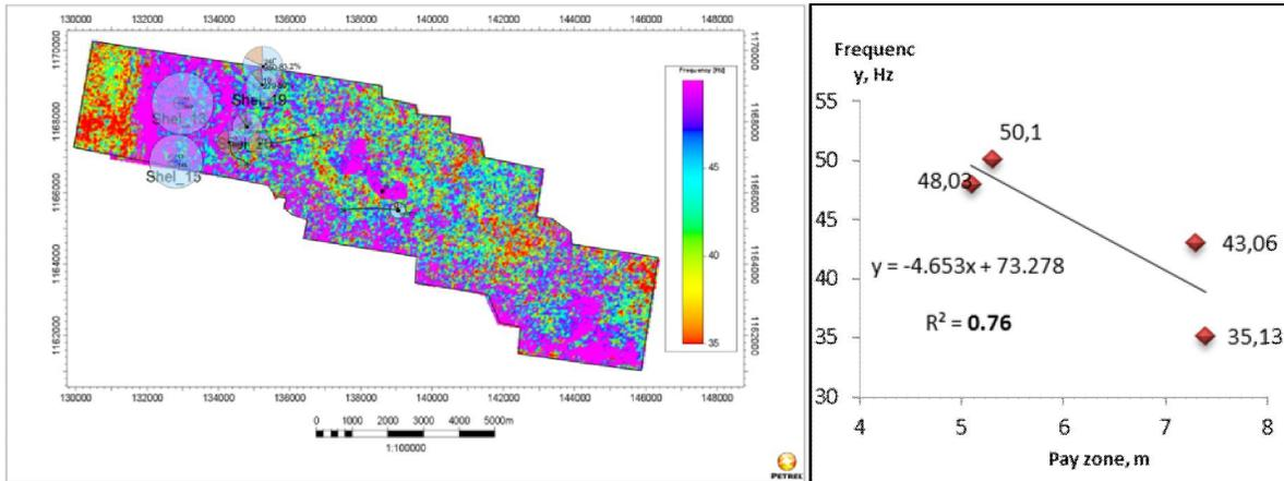
**Figure 11.** The instantaneous frequency time slice at 10 ms below the top of Domanik formation
