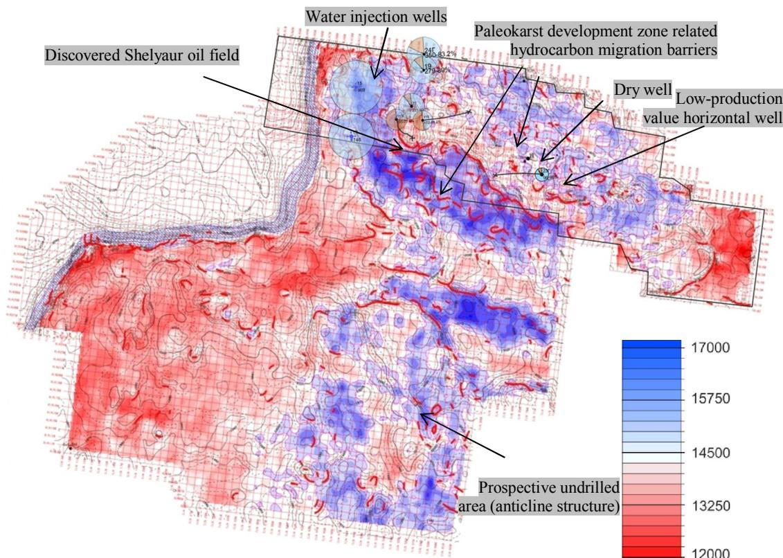
**Figure 10.** The impedance time slice at 15 ms below the top of Domanik formation.
