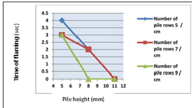
Figure (10): Effect of pile height and number of pile rows / cm for samples made of pile yarn material polypropylene 100% on time of flaming
