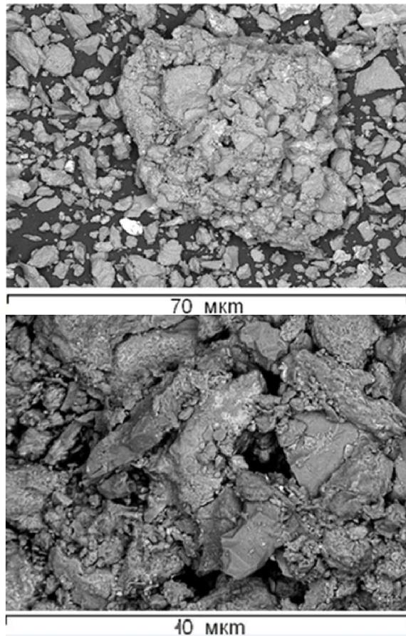
**Figure 3. Obtained aggregate. Mixture of Birkachan and Tsokol**
