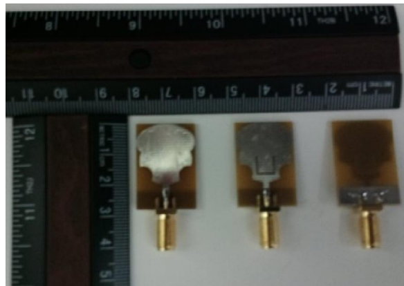
Figure 8. The prototype of the proposed antenna with and without slot.
