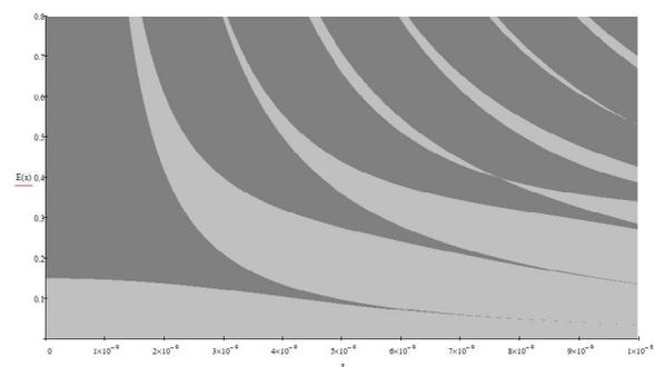
**Fig. 2. Dependence of superstructure energy levels on the value of transition period of gallium arsenide superstructure  $x$  [5]**
