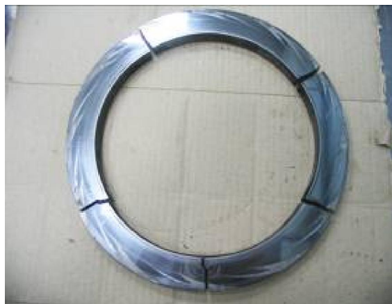
Figure 8: Vibration damage of seal ring
