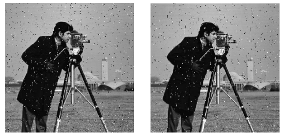
a- Code rate =1/2, K=3 b- Code rate =1/2, K=5.
