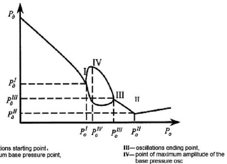
**Fig.1. Characteristic pressures on a typical dependence plot of the  $P_d$  ( $P_0$ )**
