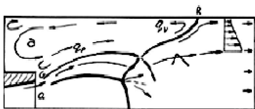
Fig. 4. Internal separation flow in the canal
