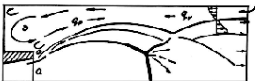
Fig. 5. Internal separation flow in the channel. The bottom area is open. Legend - as in Figure 4
