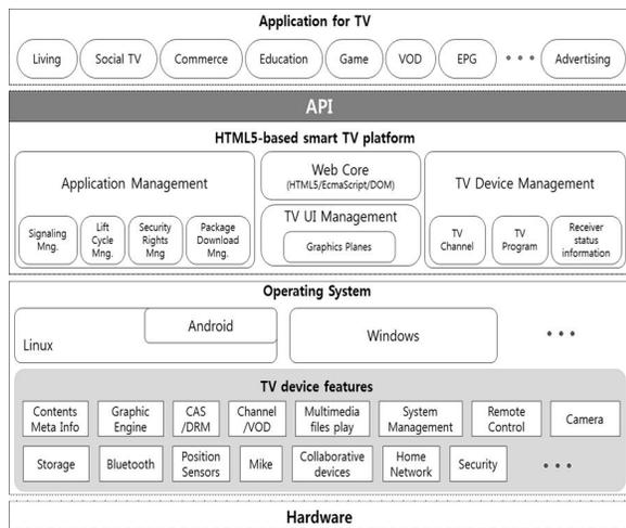
Figure 2. Smart-TV receiver platform architecture
