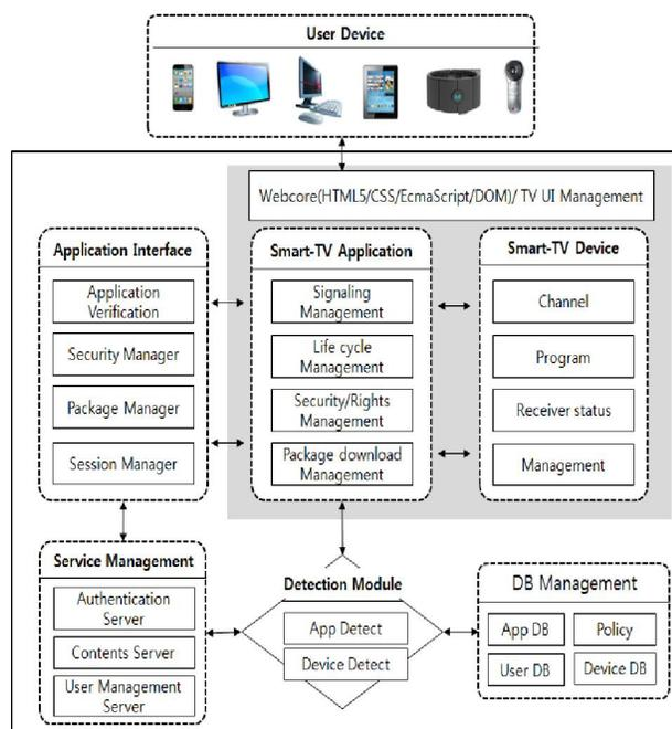
Figure 3. Structure of proposed system
