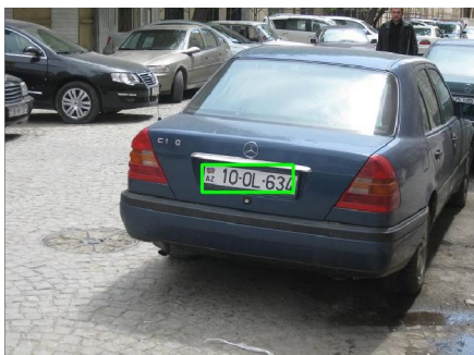
Figure 18. The extraction result of a tilted license plate
