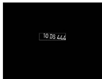
Figure 10. Plate area extracted after the verification of target area
