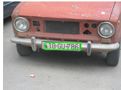
Figure 15. The extraction result from a big license plate
