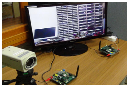
Figure 14. Test configuration of Wi-Fi video transceiver
