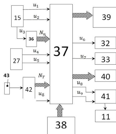
**Figure 9. Structure of a hardware component of the volumetric fuel consumption measuring system**
