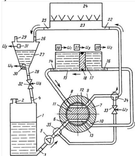
**Figure 2. Volumetric flow measurement system of a diesel engine (stable condition 1).**
