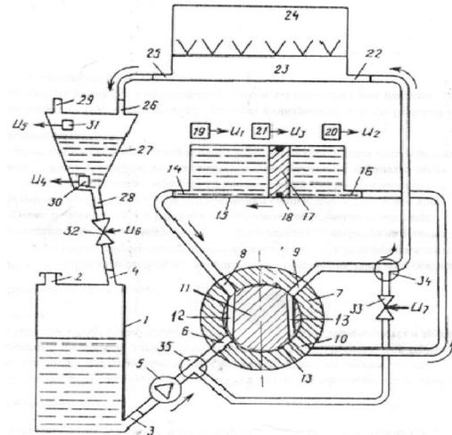
**Figure 3. Volumetric flow measurement system of a diesel engine (stable condition 2).**
