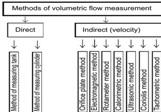
**Figure 1. Classification of volumetric flow measurement methods**
