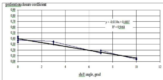
**Fig. 2 – Perforation closure coefficient in dependence of the shift angle value of the model cast bar from lead alloys (Fisher's test =0.91)**
