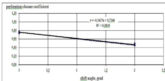
**Fig. 3 – Perforation closure coefficient in dependence of the shift angle value of the model cast bar from aluminium alloys (Fisher's test =0.98)**
