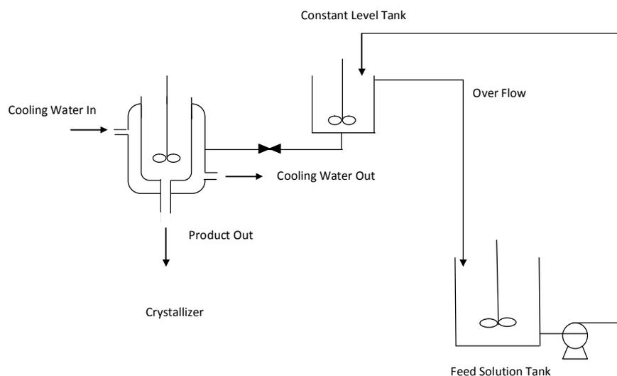
**Figure 1.** Schematic diagram of the crystallization system
