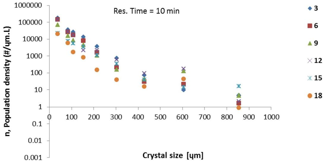
Figure 6. Population density vs. average crystal size at different degree of super saturation
