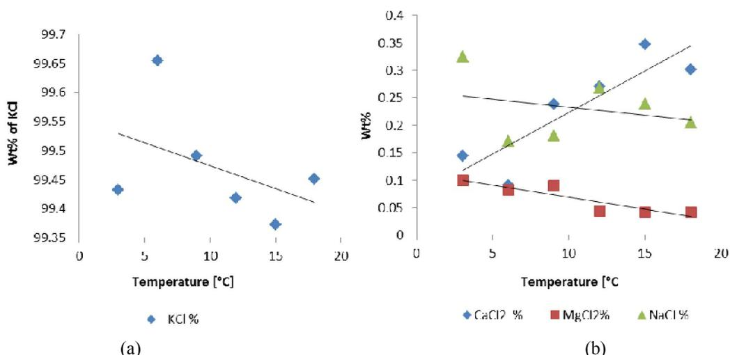
**Figure 2.** (a) Wt. % of KCl vs. degree of supersaturation, (b) Wt. % of CaCl<sub>2</sub>, MgCl<sub>2</sub>, NaCl vs. degree of supersaturation
