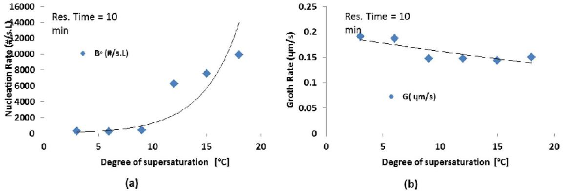
Figure 3. (a) Nucleation rate vs. degree of supersaturation, (b) Growth rate vs. degree of supersaturation
