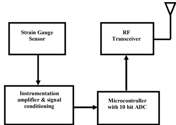
Figure 2: A wireless sensor node functional block diagram
