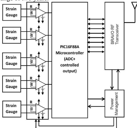
Figure 4: Wireless sensor node circuit diagram
