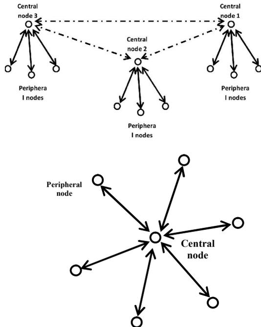
Figure 1: Wireless sensor network topology used; A. Star network and B. Two-peer network.
