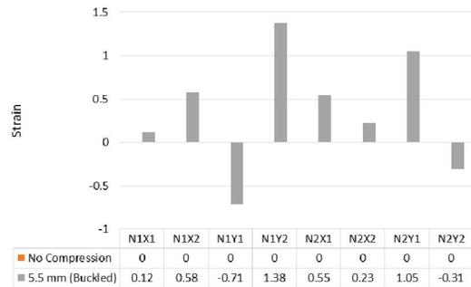
Figure 10: Strain in various gauges during buckling along the length
