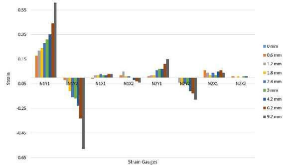
Figure 8: Strain at various locations during radial loading
