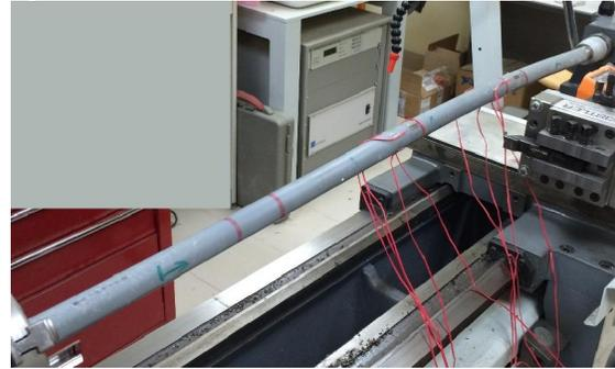
Figure 7: Experimental setup for axial compression
