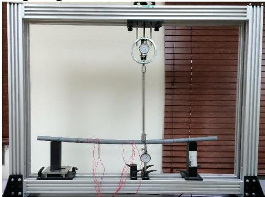
Figure 6: Experimental setup for radial bending
