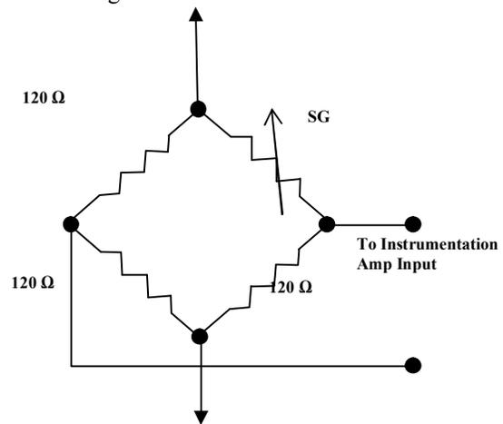
Figure 3: Quarter-bridge strain gauge circuit
