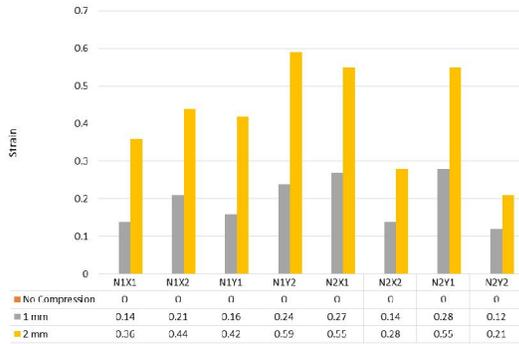
Figure 9: Strain in various gauges during axial compression
