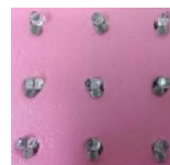
Figure 4. The simple 3×3 LEDs electronic drawing board.
