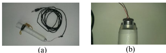
Figure 1 The signals acquisition components of the measurement devices. (a) is shown as whole device and (b) focuses on the zoom in picture of simple microphone.
