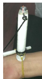
Figure 3. The measurement setup. The pulse sensor is fixed on the wrist and connects to the laptop.
